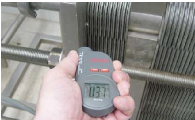
Figure 31: Using a simple laser thermometer 41
