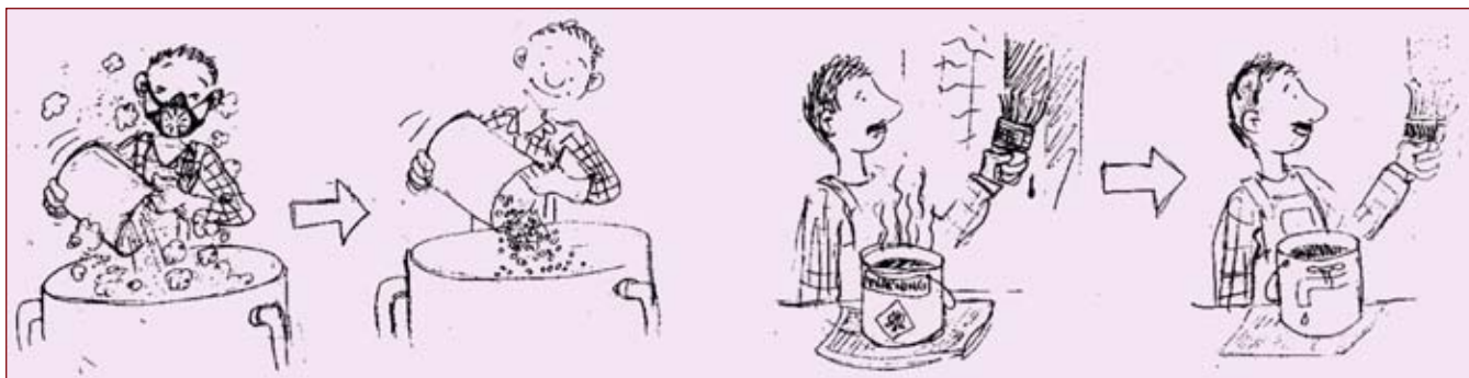
Figure 46: Using pellets instead of powders and using water-based paint instead of oil-based 95
